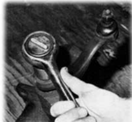
Jack up the car and support it safely. Remove the large nut securing the pitman arm, then, using a puller, remove the arm.
