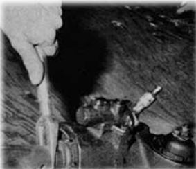
Pry the pot coupling off the steering box. A pickle fork works great for this. If you have a column shift, disconnect the linkage from the lever protruding from the base of the column jacket. Take off that last nut, unplug the electrical connectors, and remove the column assembly.
