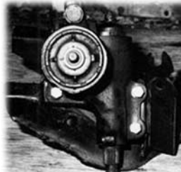
Remove the three special bolts securing the box (chuck) to the K-member. Disconnect the hoses and pull the box up and out. On most cars you'll have to unbolt the driver's side motor mount and raise the engine a few inches to gain enough clearance.
