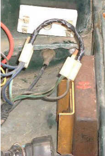
This photo shows the ballast resistor being bypassed, and the Chrysler Electronic Unhooked.
