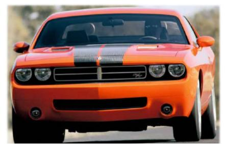
and 21 inch wheels on back), and runs the quarter mile in 13 seconds flat; top speed is 174 mph (limited by wind resistance), while gas mileage is estimated at 14 city, 20 highway, very good compared with the original
